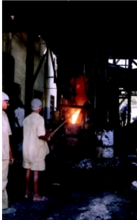
Figure 5 Conventional cupola in operation
