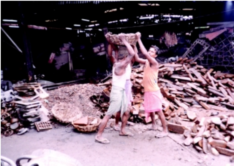
Figure 8 Manual charging with baskets
