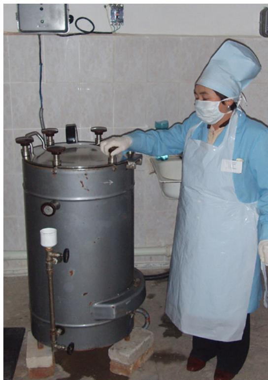
*Waste is safely disinfected under high pressure in the autoclave*
